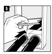
Insert a stayplate on top of every finished row of modules.
