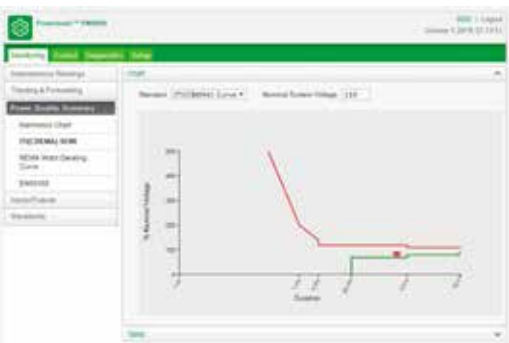
PowerLogic PM8000 series CBEMA web page sample
